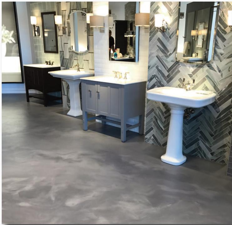
Smooth Duo, an epoxy, liquid-rich, free-flowing formulation incorporates rapidly renewable raw materials. As shown: installed on a concrete slab substrate with primer, Smooth Duo in Halifax Rain, an aromatic urethane handcrafted finish with a matte top coat.
